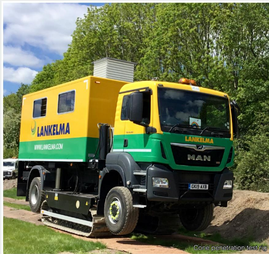
Cone penetration test rig
