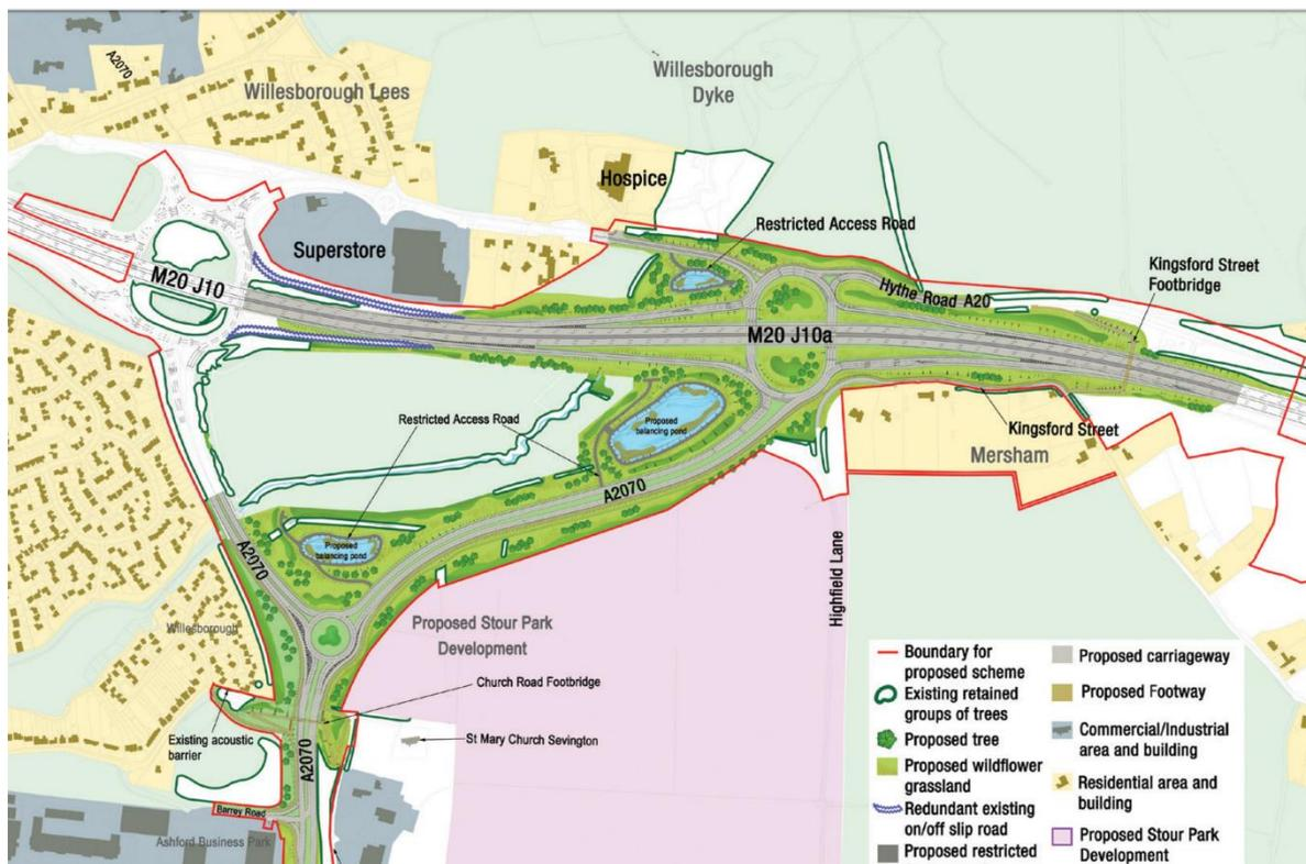
Drivers will be able to access the M20 travelling eastbound using the new A2070 link road and M20 J10a. Drivers travelling westbound will also be able to exit the M20 at the new junction 10a and travel towards Ashford using the A2070 link road.
