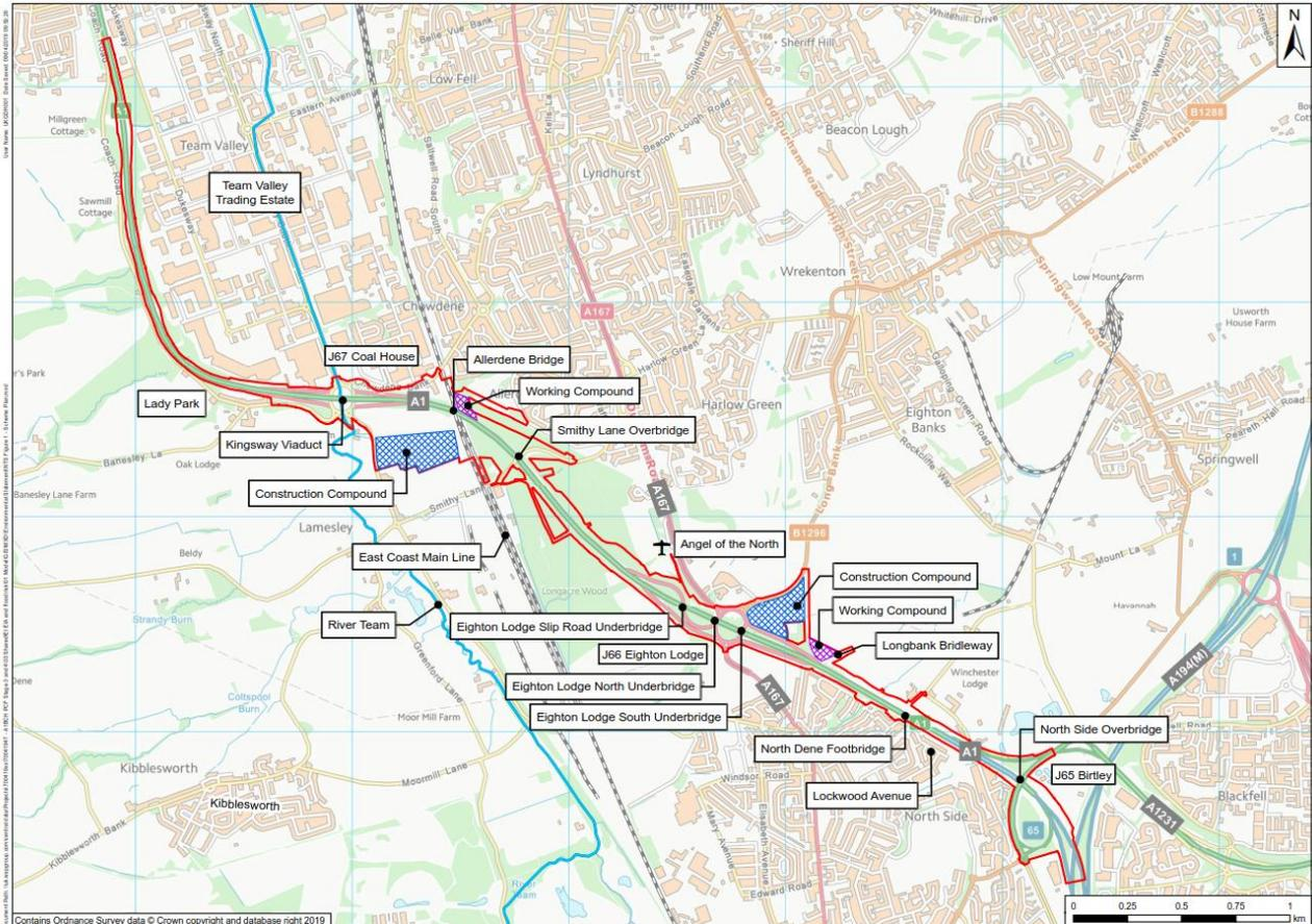
The existing Allerdene Bridge would be demolished, and the replacement bridge would be located approximately 40 metres to the south of the current structure between junction 67 (Coal House) and Smithy Lane Overbridge.
